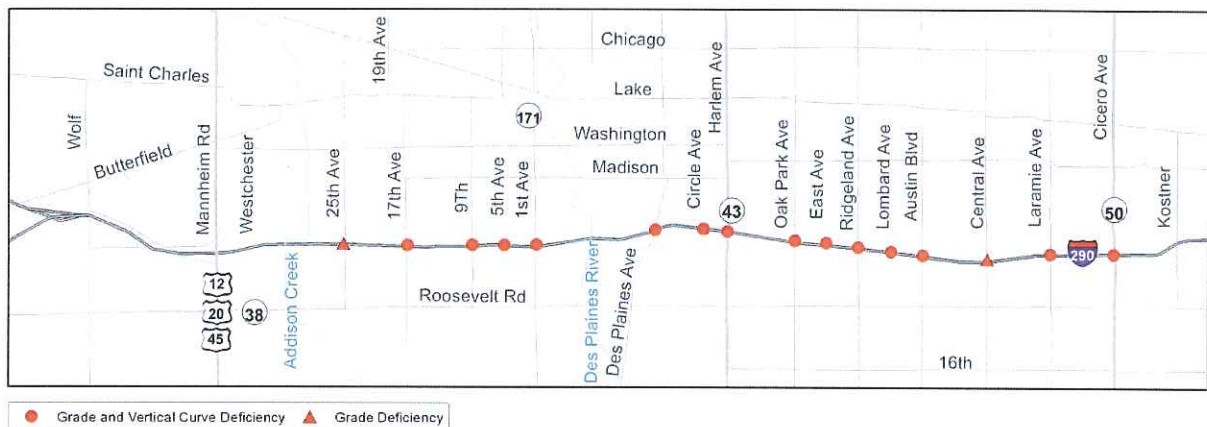
Figure 1-14 - Existing Crossroad Vertical Geometry Deficiencies
