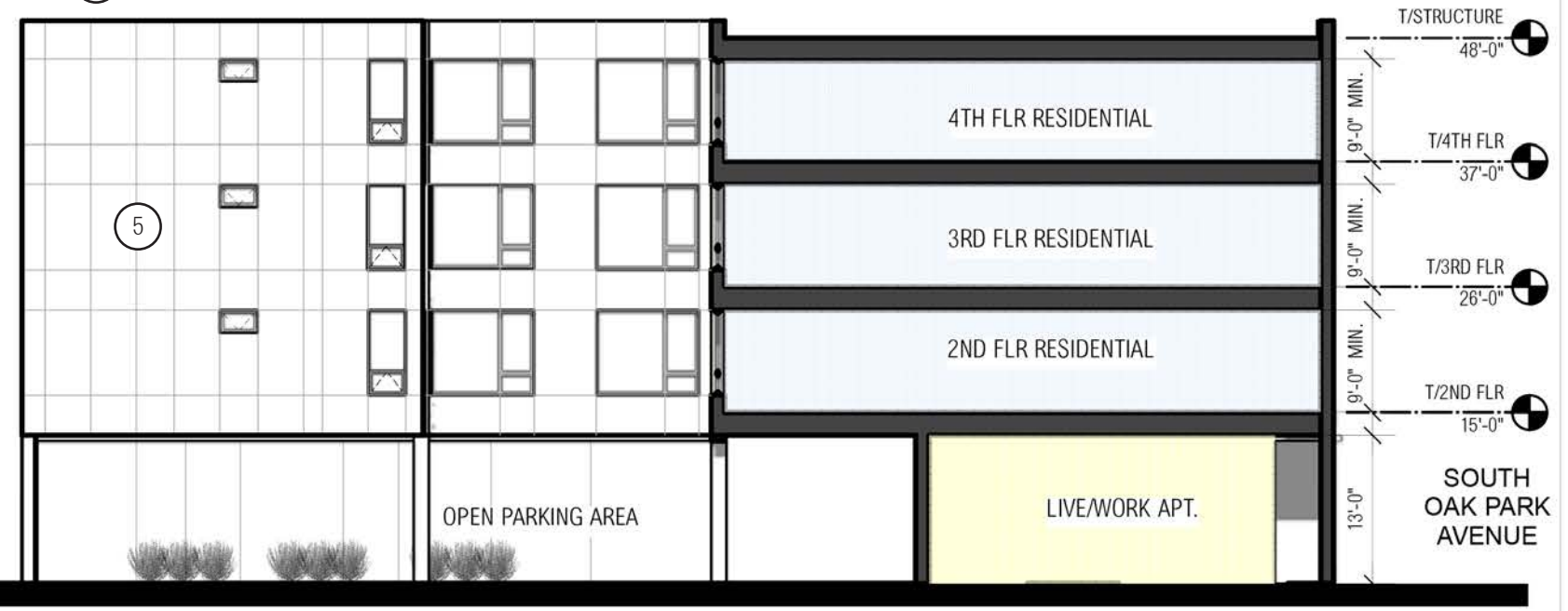
4 SOUTH EXTERIOR ELEVATION / SECTION Scale: 1/16" = 1'-0" 0 10 20 FT
