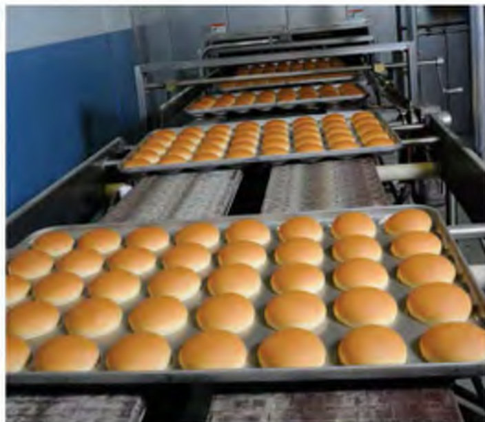
Freshly baked hamburger buns leave the oven and head to the spiral cooler.
