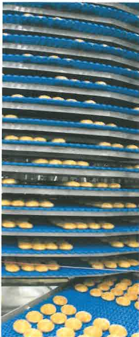
▲ Buns cool after baking by traveling through a multitier ambient-temperature spiral conveyor at Turano Florida Bun, Orlando, FL.
