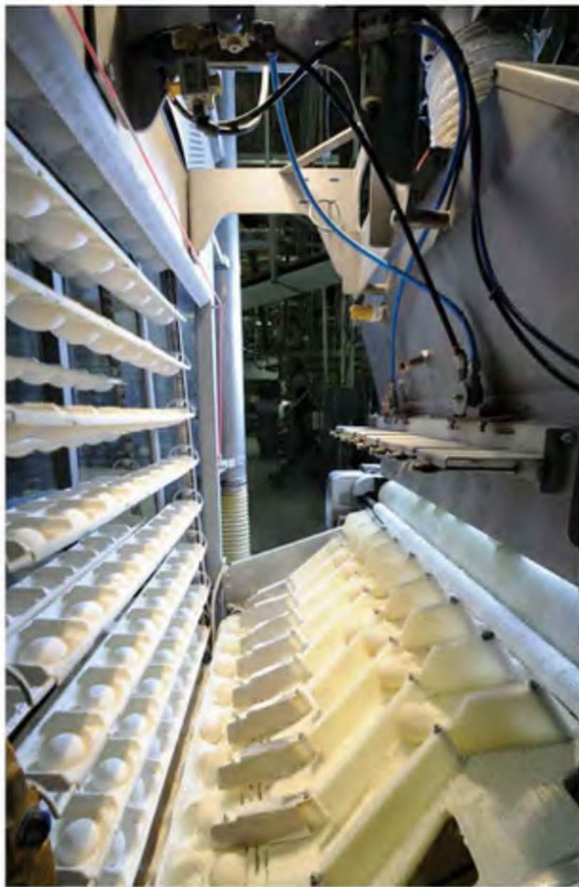
Dough pieces tumble from the divider and rounder bars and into the intermediate proofer.
