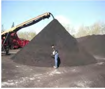
IDOT Reclaimed asphalt shingles in Illinois for use in sustainable warm asphalt mix
