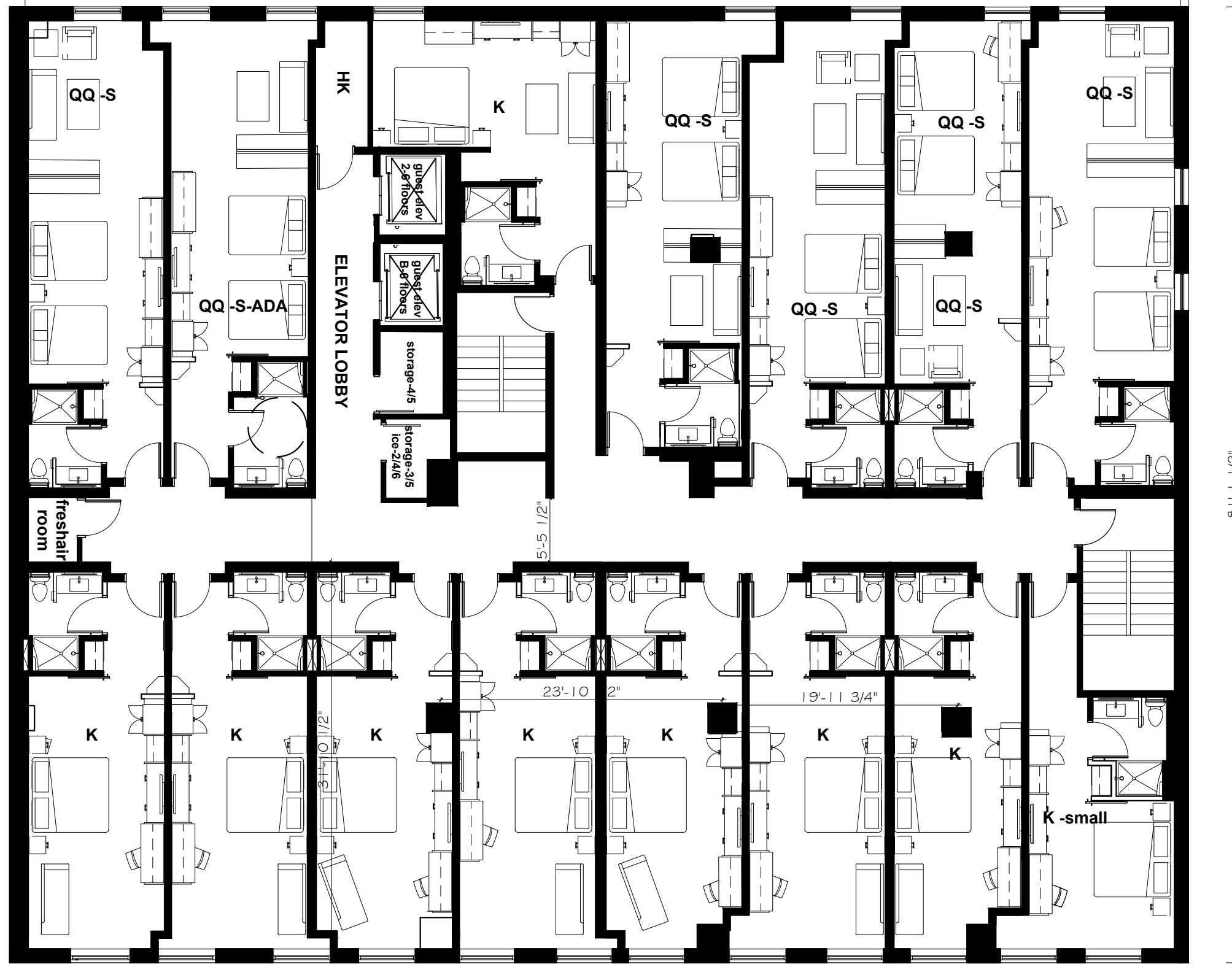
3RD/4TH/5TH FLOOR - 15 GUEST ROOMS PER FLOOR - FLOOR AREA: 8025 SF : 8- KINGS, 1-KING SUITE , 5- QQ SUITES- 1- QQ ADA SUITE
