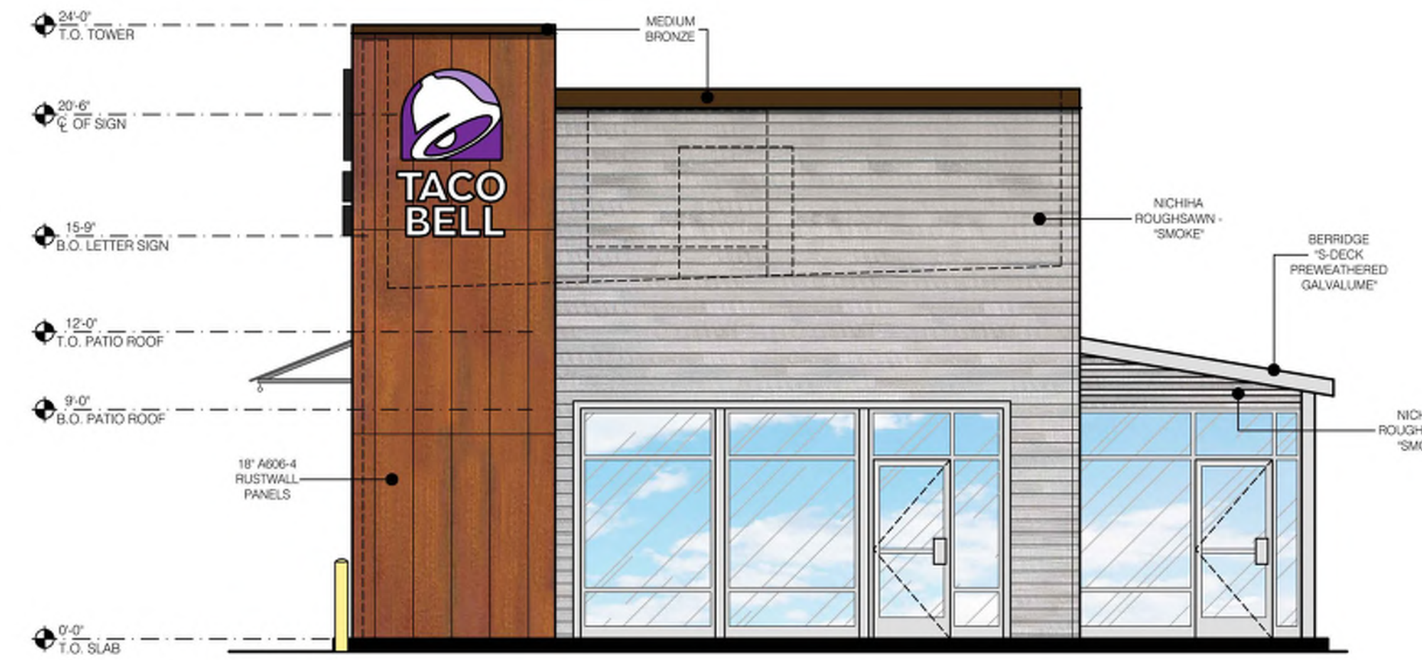
EAST ELEVATION 3/16" = 1'-0" B
