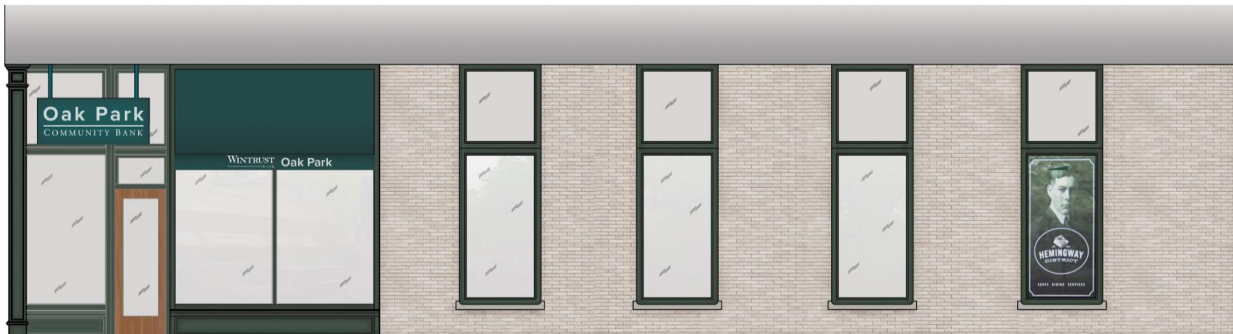
5 LAKE STREET ELEVATION WITH AWNING & SIGNAGE SCALE: 1/4" = 1'-0"
