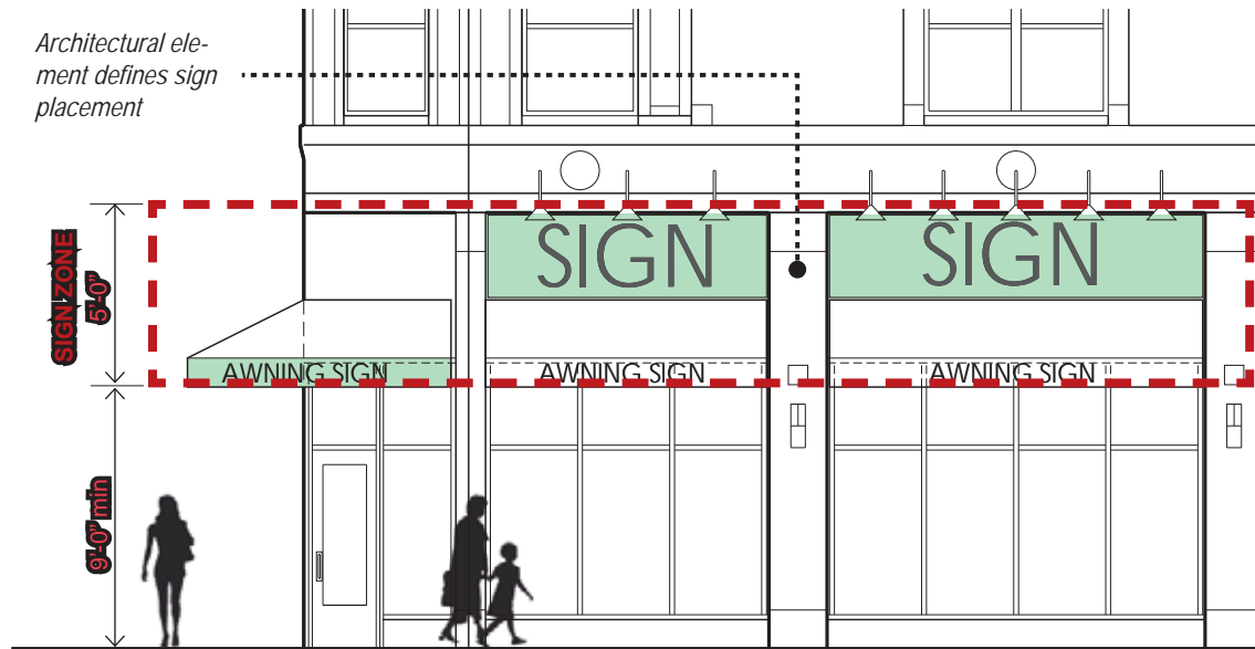
Figure 7.35: Ideal Arrangement for Storefront Signage
