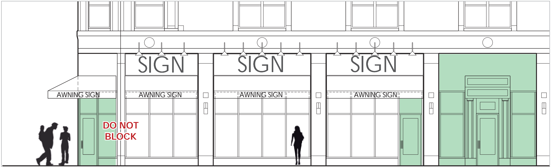
Figure 7.37: Ideal Arrangement for Placement of Entrances
