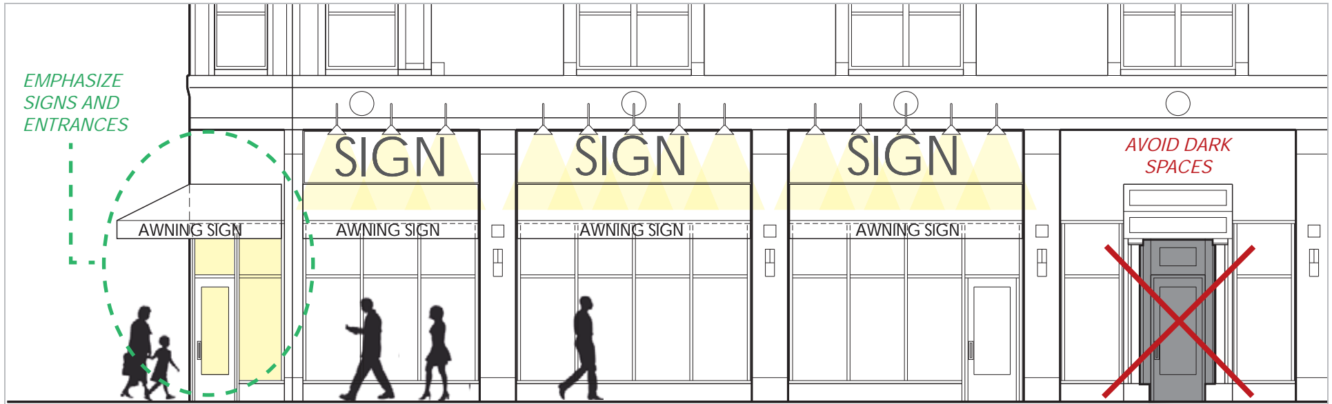
Figure 7.39: Ideal Arrangement for Storefront Lighting
