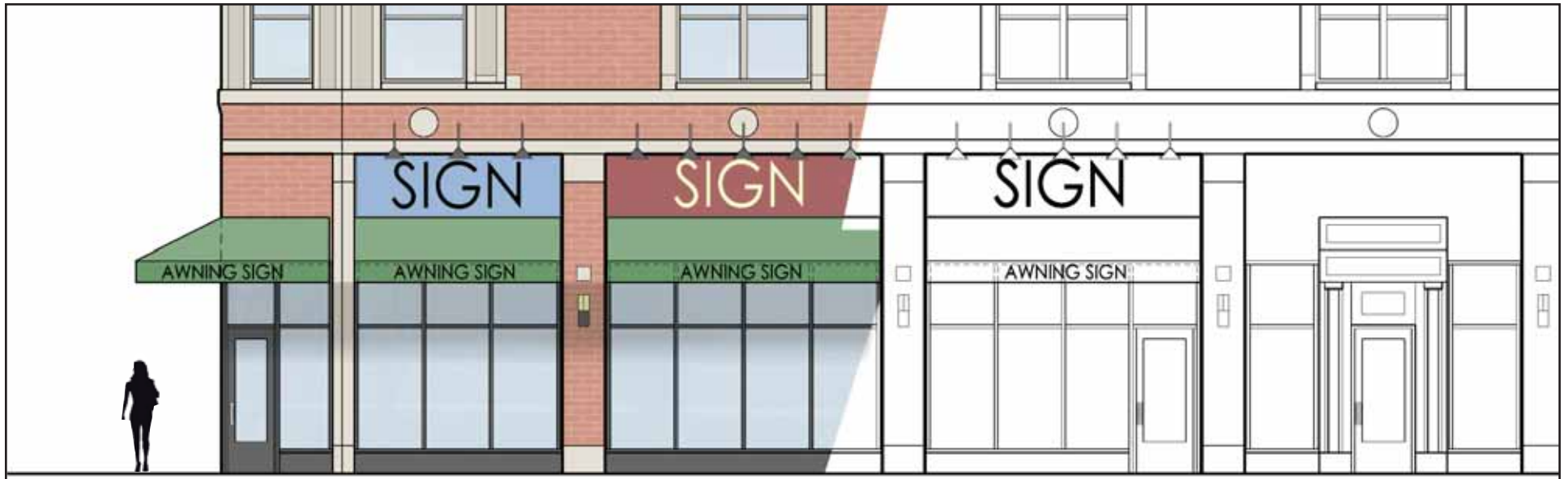
Figure 7.40: Consistent Building Colors and Materials on Retail Facades
