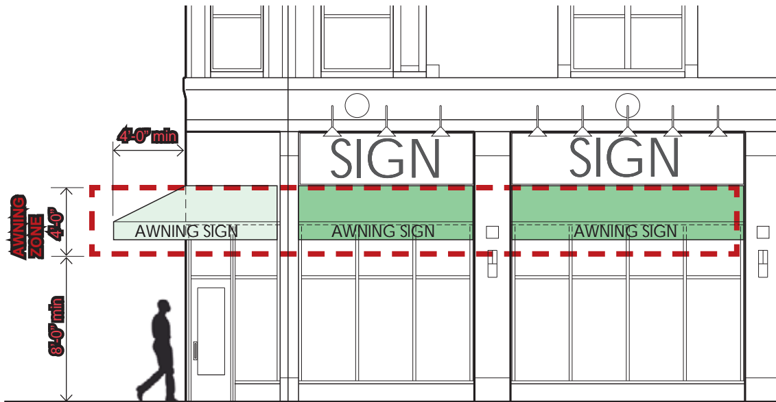
Figure 7.33: Ideal Arrangement for Awning Placement
