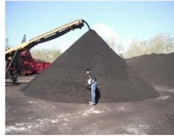
IDOT Reclaimed asphalt shingles in Illinois for use in sustainable warm asphalt mix
