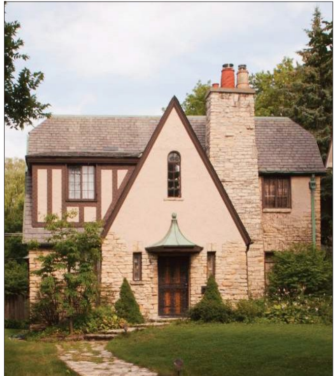
Stucco is often used in addition to other materials as a wall material. In this example, it is combined with limestone and half-timbering.
