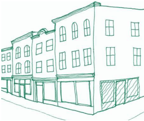
The entrance of the corner building is oriented towards the perpendicular street and is inappropriate.
