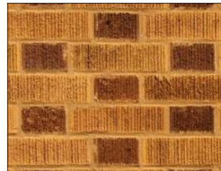
Wire Cut Brick - A hard, dense, fired-clay, regularly shaped building component, with a ridged surface.
