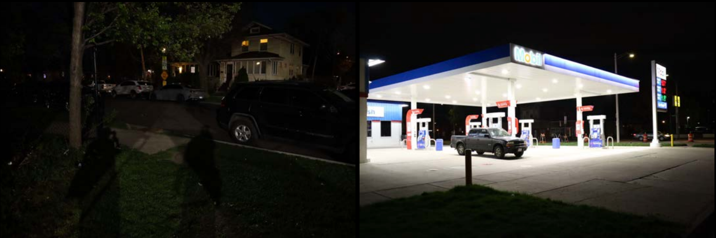
Figure 13: Significant light trespass from the BP station can be seen on the home across the street (left). Light levels under the canopy at a gas station on Madison (right) peaked at 790 lux. The IES recommended standard is 135 lux. Positively, the station does not use lights exterior to their canopy.
