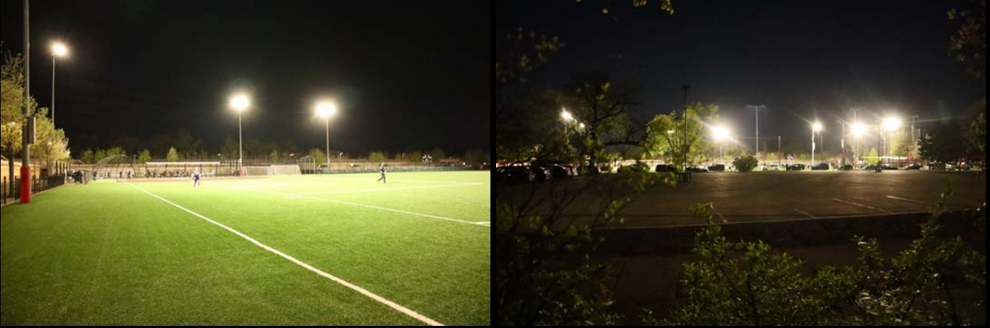
Figure 10: Glare from high intensity and unshielded lights at Ridgeland Commons field (left). View of the field lights as seen from the home on N Elwood (right).
