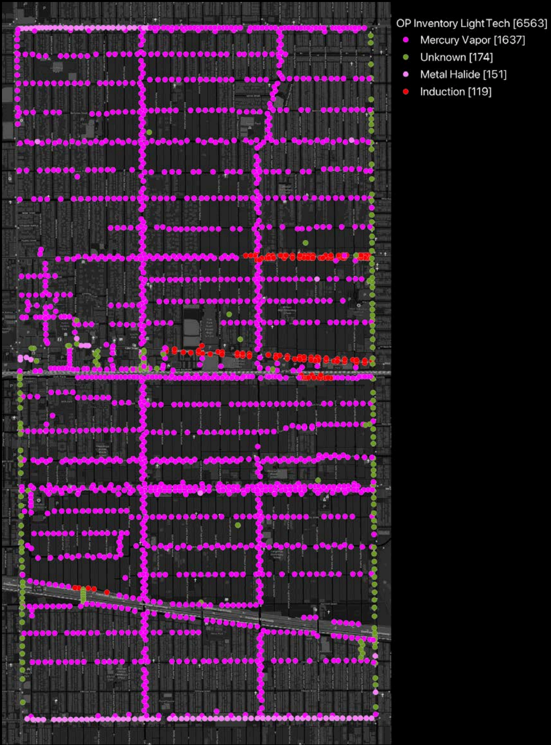
Figure 20: Location of VOP Light Technology Inventory exceeding recommended color temperature (>3000K)
