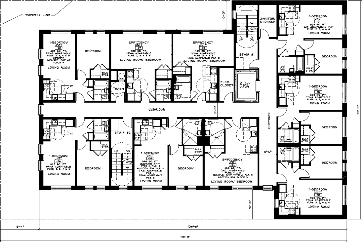
1 TYPICAL FLOOR PLAN (FLOORS 2, 3, 4 & 5) SCALE: 1" = 10'-0"
